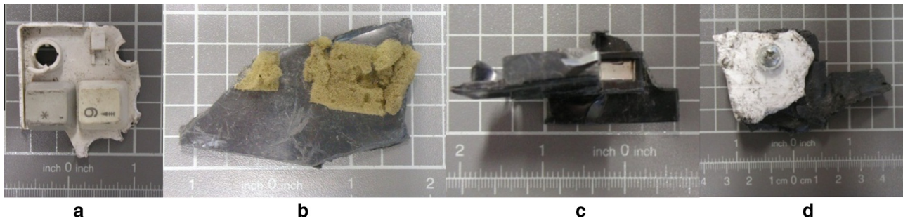
Photo 2. (a) Polymer/polymer clipping, (b) polymer/foam sticking, (c) polymer/metal insertion and (d) polymer/polymer/metal screwing.
