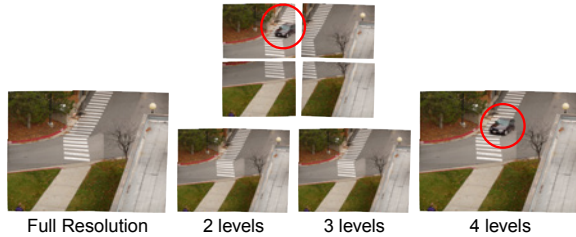
Figure 1: An example case where a deep hierarchy for Hierarchical Graph Cuts produces poor results. A car that appears in only one of the input images (top) causes a region with high energy which a pixel based energy will avoid. The results for up to 3 levels are good. At 4 levels, in the coarse solution, the car is small enough for the seam to pass through it. The dilation parameter (10 pixels in the typical case) is not large enough to exit this local minima in the refinement stages.
