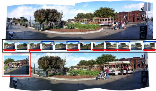
Fig. 3. Support for the interactive adding and removing of images while providing a fast preview enables a user to explore the space of all panoramas for any image dataset. For example, a user can make multiple distinct panoramas (top: blue, bottom: red) from this single dataset where, for example, the departing cable car (bottom inset) appears only in the one panorama.
