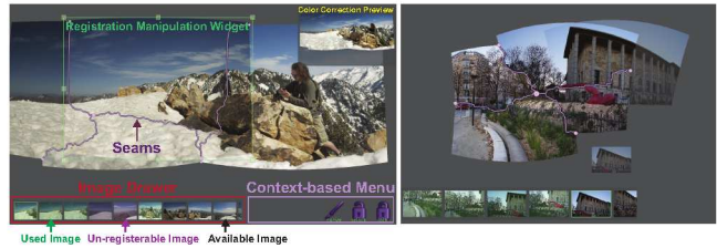
Fig. 14. (left) Annotated screenshot of our interactive system. (right) When a user selects an image, a preview of the registration is provided based on the highest confidence pairwise homography.
