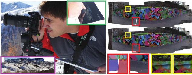
Fig. 2. Our new methods for interactive creation of panoramas enable, for the first time, in-the-field acquisition of professional quality panoramas with no assumptions on the structure of the images or specialized hardware; (inset green) a computer coupled with a tablet device provide full editing in-the-field; (inset purple) a panorama created from an in-the-field deployment of the prototype software. In-the-field editing can allow a user to potentially identify missing data during acquisition and acquire new images to fill in gaps (inset red) and/or fix registration misalignment on the spot (inset yellow) for this panorama. (52.9 megapixel, 15 images).
