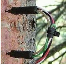
(a) Sap flow sensors: Granier probes are composed of two thermocouple needles.
