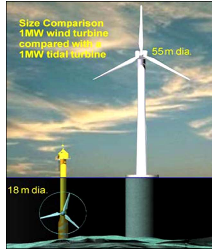
Fig. 5. Tidal turbine against an offshore wind turbine [Marine Current Turbine (© MCT, Bristol, U.K., www.marineturbines.com)].
