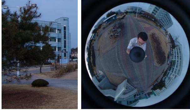
Fig. 1. Compared to traditional perspective cameras (left), catadioptric systems (right) can gather much more information from the environment.
