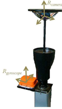
Fig. 12. The coordinate systems of the camera and the gyroscope
