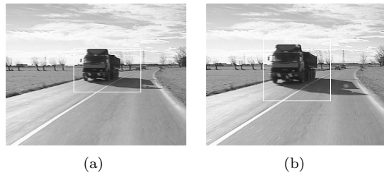
Fig. 6. Obstacle detection on the road sequence. \alpha = 8 , \beta = 100 , \epsilon = 1.2 . (a) t = 66 , (b) t = 70 .
