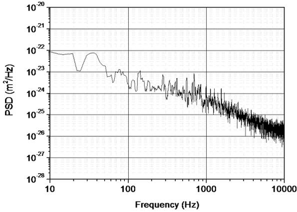
FIG. 4 Power spectral density (PSD) of the vibration measurements on the mirror in a static configuration. The estimated noise is  $600 \text{ fm}\cdot\text{Hz}^{-1/2}$  @1 kHz and  $150 \text{ fm}\cdot\text{Hz}^{-1/2}$  @10 kHz. The flicker noise is not reached at 10 kHz but the data acquisition board is limited for higher sample frequencies.
