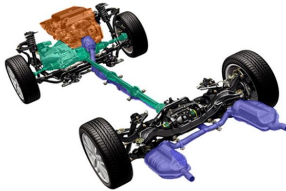
Figure 7 Powertrain system of a modern automobile (Akehurst, 2007)
