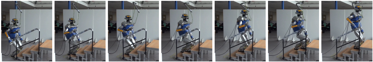
Fig. 5: Exp.2 - Climbing the stairs of 15cm height by using the handrail.
