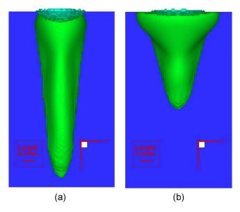
FIG. 6. Calculated weld pool profiles at 31 ms welding time during laser welding under variable ambient pressure (2 kW, 3 m/min). (a) Vacuum and (b) atmospheric pressure.
