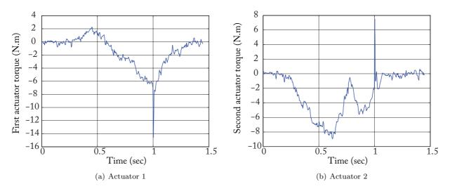
Fig. 16 Input torques measured for the five-bar mechanism crossing the Type 2 singularity locus at  $t_s = 0.75$  sec respecting the dynamic criterion (62)
