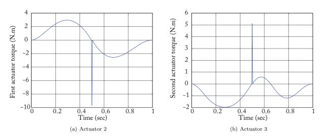
Fig. 20 Input torques simulated for the Tripteron crossing the LPJTS singularity locus at  $t_s = 0.5$  sec without respecting the dynamic criterion (65)
