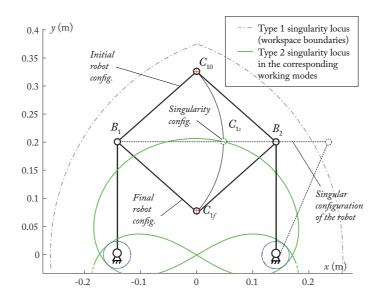
(b) Equivalent trajectory of the five-bar mechanism
