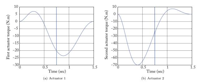
Fig. 11 Input torques simulated for the five-bar mechanism crossing the Type 2 singularity locus at  $t_s = 0.75$  sec without respecting the dynamic criterion (62)
