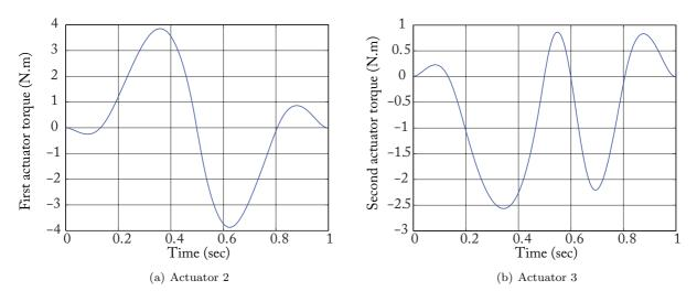
Fig. 21 Input torques simulated for the Tripteron crossing the *LPJTS* singularity locus at  $t_s = 0.5$  sec with respecting the dynamic criterion (65)
