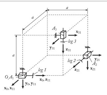
Fig. 17 Kinematic description of the actuated prismatic joint arrangement for the Tripteron
