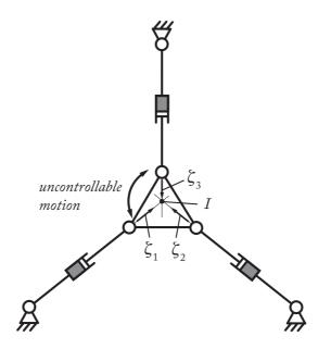
Fig. 2 Example of Type 2 singularity of a 3-RPR planar parallel robot (grey joints denote actuated joints): in that case, the platform has one uncontrollable motion which is an instantaneous rotation around the point I
