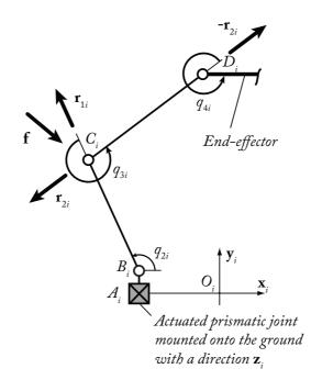
(b) Kinematic architecture of the leg i
