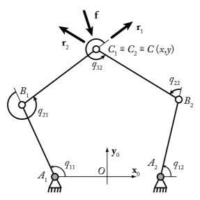
Fig. 4 Kinematic chain of the five-bar mechanism
