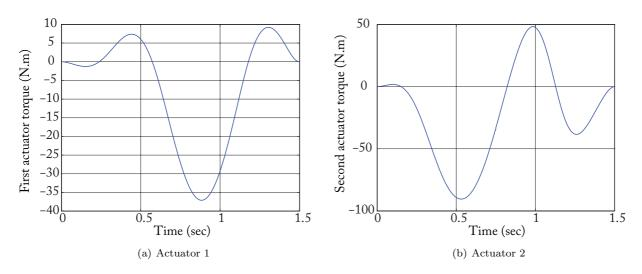
Fig. 12 Input torques simulated for the five-bar mechanism crossing the Type 2 singularity locus at  $t_s = 0.75$  sec respecting the dynamic criterion (62)
