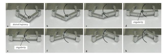
Fig. 23 The five-bar mechanism tracking the trajectory respecting the dynamic criterion (65)
