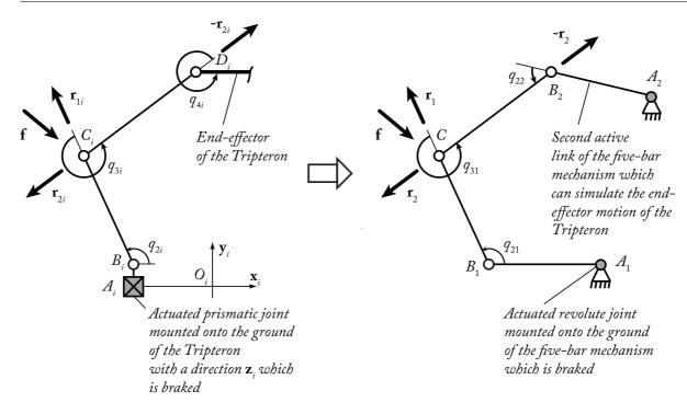
Fig. 18 Equivalence between the leg i of the Tripteron and the five-bar mechanism architecture
