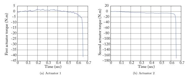
Fig. 15 Input torques measured for the five-bar mechanism crossing the Type 2 singularity locus at  $t_s = 0.75$  sec without respecting the dynamic criterion (62)
