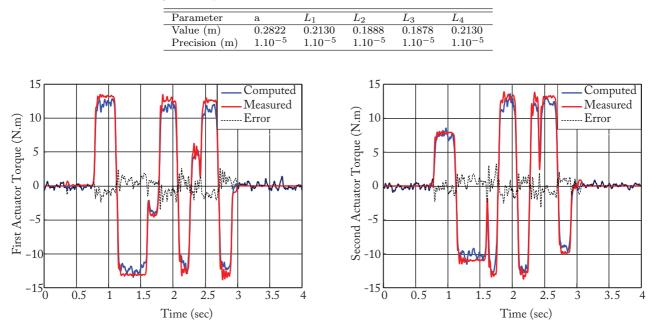
Fig. 9 Verification of the identified dynamic model
