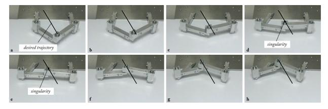
Fig. 14 The five-bar mechanism tracking the trajectory respecting the dynamic criterion (62)
