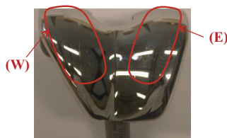
Fig. 1. The 2 wear zones of analysis.
