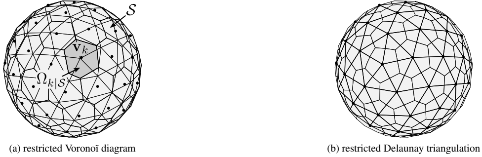
Figure 1: Restricted Voronoi diagram and Delaunay triangulation, with \mathcal{S} being a sphere in \mathbb{R}^3 .
