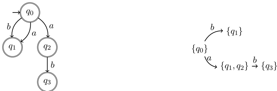
Figure 1: An example of non-flankable NFA (left) and its associated Rabin-Scott power-set construction (right).
