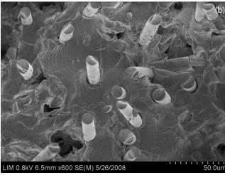
FIG. 15. (a) SEM of fatigue failure surface in the subskin position of a sample tested in AFF at 10 Hz,  $\varepsilon_0=0.017,~\sigma_{\rm max}=102$  MPa, 20  $\mu$  scale. (b) SEM of fatigue failure surface (core position) of a sample tested in AFF at 10 Hz,  $\varepsilon_0=0.017,~\sigma_{\rm max}=102$  MPa 50  $\mu$  scale.
