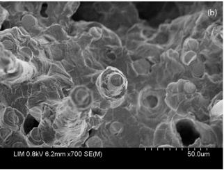
FIG. 13. (a) SEM of fatigue failure surface in the subskin position of a sample tested in TTF at 20 Hz,  $\sigma_{\rm max}=66$  MPa, 10  $\mu$  scale. Sheath of matrix is observable around the fiber. (b) SEM of fatigue failure surface of a same sample tested as in (a) (TTF at 20 Hz,  $\sigma_{\rm max}=66$  MPa) 50  $\mu$  scale.
