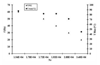
FIG. 12. Frequency variation (20–60 Hz) and maximum temperature versus the number of cycles at fracture,  $\sigma_{\rm Max}=72$  MPa– $\sigma_{\rm Min}=21$  MPa (R=0.3).
