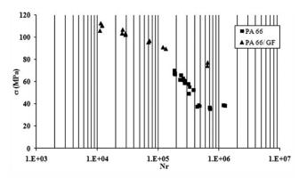
FIG. 10. Wohler curves of PA 66 and PA66/GF in AFF tests at 10 Hz.
