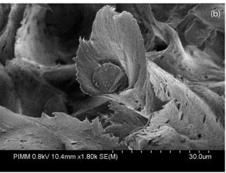
FIG. 14. (a) SEM of the failure surface after a tensile test at room temperature. (b) SEM of the failure surface after a tensile test at 90°C.
