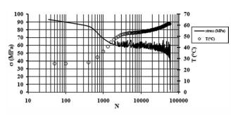
FIG. 4. Induced stress and surface temperature of a PA66/GF sample tested at 10 Hz in AFF  $\varepsilon_0=0.017$ , versus the number of cycles.
