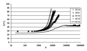
FIG. 11. Surface temperature variation induced by self-heating during TTF test,  $\sigma_{\rm Max}=72$  MPa- $\sigma_{\rm Min}=21$  MPa (R=0.3) at various frequencies (20–60 Hz).
