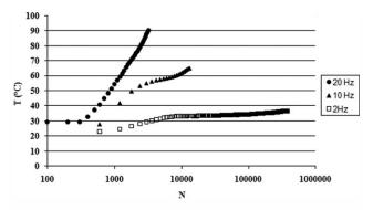
FIG. 6. Surface temperature variation during AFF tests at 2, 10, and 20 Hz, correspond to  $\varepsilon_0=0.019.$
