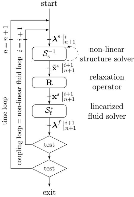
Figure 1: coupling algorithm
