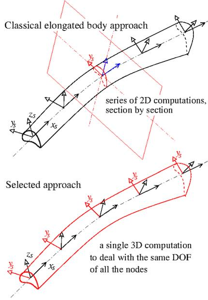
Figure 2: computation of the added-mass operator for an elongated body
