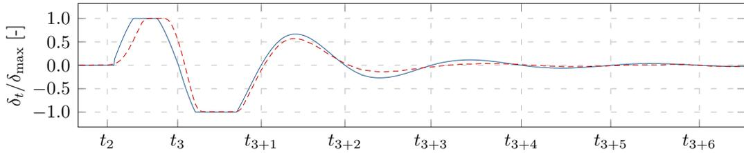
**Figure 5:** Starboard fin angle – Active fins : - - - experimental tests, — present work
