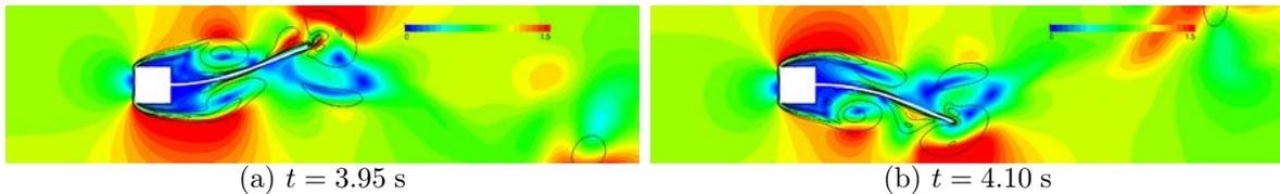
**Figure 8:** 2D flexible membrane – Dimensionless velocity field and iso-lines of vorticity
