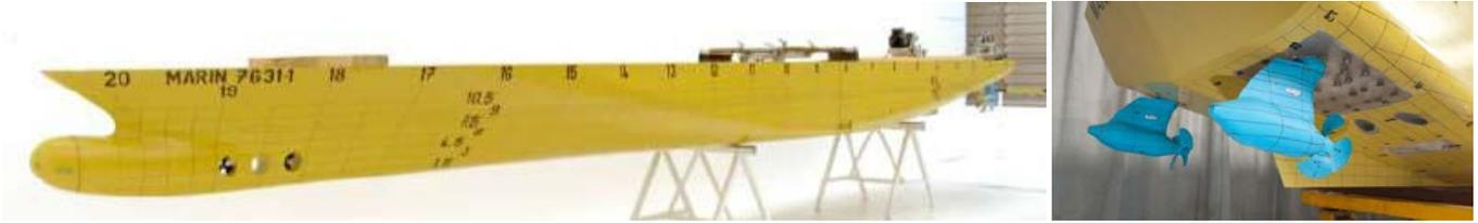
**FIGURE 1.** SHIP MODEL WITH PODED PROPELLERS.
