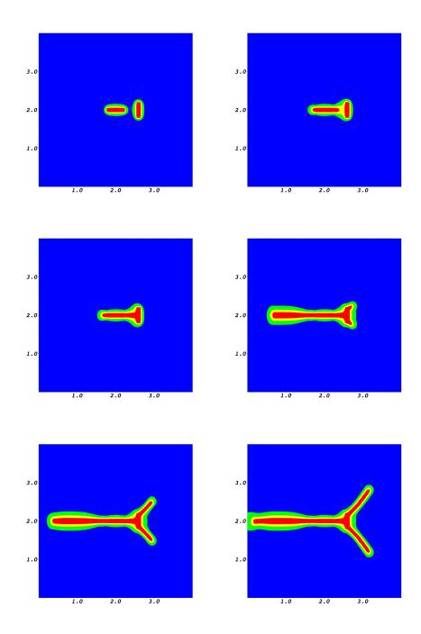
Figure 7: Example 2: Crack pattern at times T=1,6,7,20,30,50s with two fractures. Fracture 1 (the horizontal fracture) joins fracture 2 (the vertical fracture) at T=7s. The crack pattern is displayed with the help of the phase-field variable  $\varphi$ . In the crack (red colored) region  $\varphi=0$  and in the unbroken material,  $\varphi=1$ . In between  $0<\varphi<1$ , which denotes the smooth transition zone.
