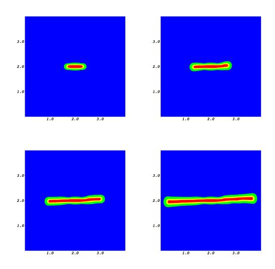
Figure 11: Example 3: Crack pattern at times T=10,20,30,50s using the phase-field variable  $\varphi$ . In the crack (red colored) region  $\varphi=0$  and in the unbroken material,  $\varphi=1$ . In between  $0<\varphi<1$ , which denotes the smooth transition zone.
