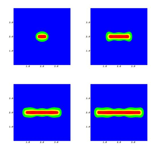
Figure 2: Example 1: Crack pattern at times T=1,10,20,30s using the phase-field variable  $\varphi$ . In the crack (red colored) region  $\varphi=0$  and in the unbroken material,  $\varphi=1$ . In between  $0<\varphi<1$ , which denotes the smooth transition zone.
