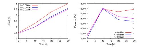
Figure 6: Example 1: Convergence studies of crack length and maximum pressure versus time on three different mesh levels. For fixed  $\varepsilon$ , we observe h-convergence in the length as well as in the pressure. In particular, we observe a pressure drop while the crack is growing. On the coarse mesh the pressure again increases while the pressure is monotonically decreasing on the two fine meshes.
