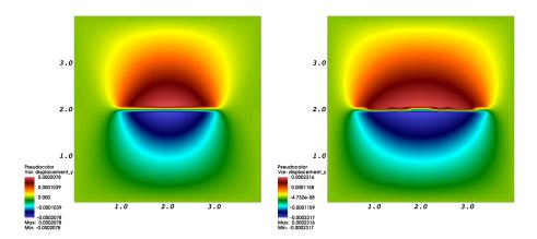
Figure 5: Example 1: y-displacement field (in m) at times T = 1, 10, 30, 40s. Here, the displacements are zero at the tips of the fracture and the highest value is obtained in the middle. As in the first example, this corresponds to the theoretical calculations of [20] in their Section 2.4.
