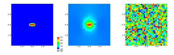
Figure 10: Example 3: Initial crack, pressure and permeability distribution
