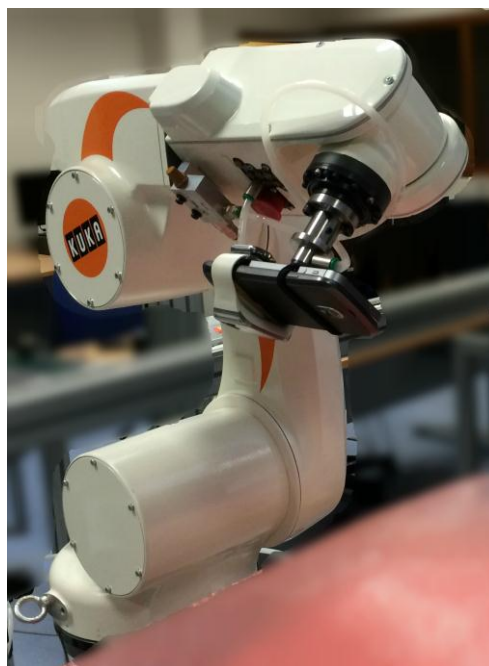
Figure 3. Picture showing the two smartphones superimposed mounted on the robotic arm.
