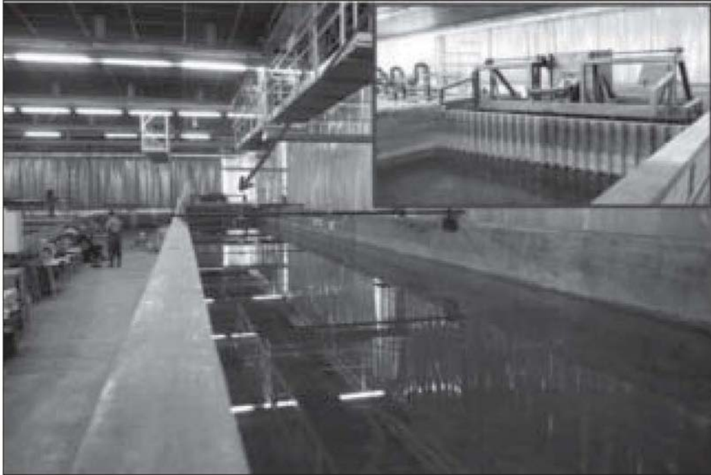
Figure 4: Side view of the wave paddle (up-right) and front view of the large wave flume at Flanders Hydraulics Research, Belgium.
