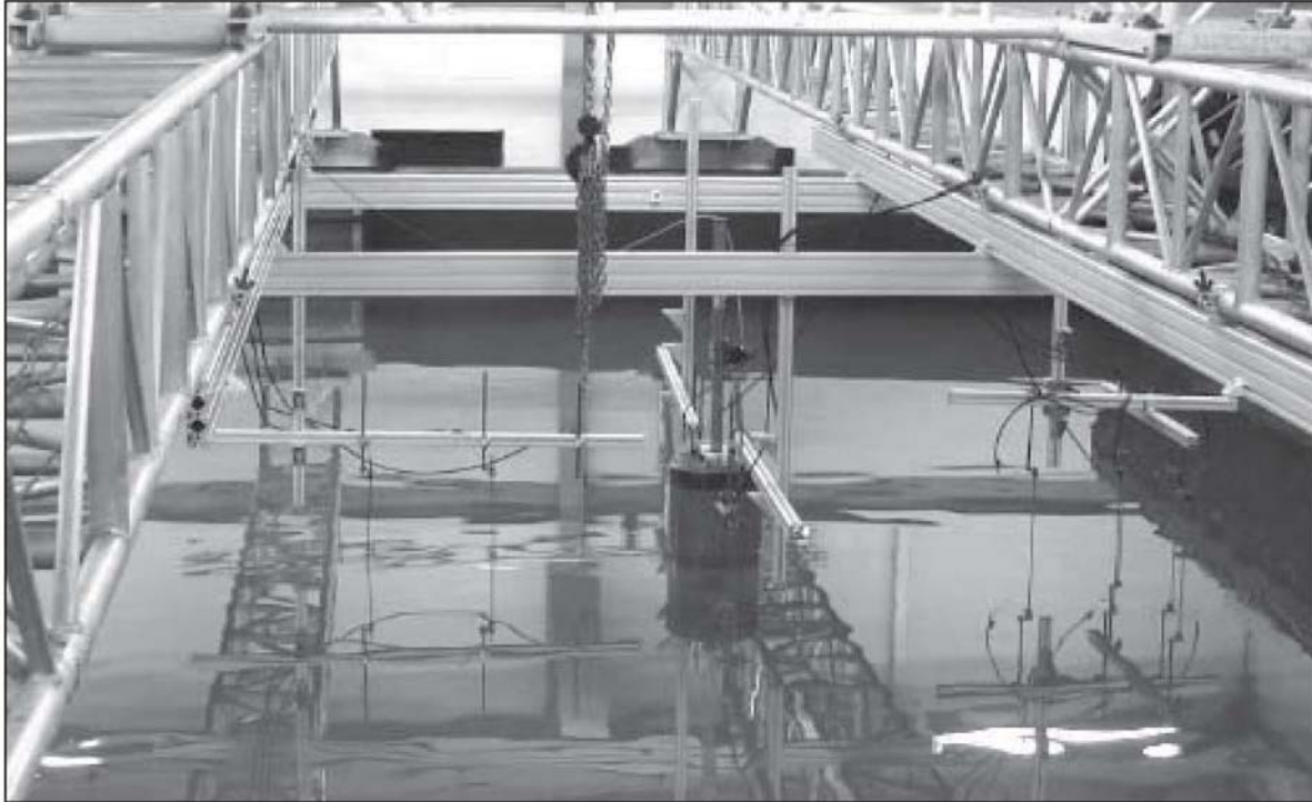
Figure 6. Side view of the developed generic point absorber WEC in the experimental set-up of the wave basin of Queen's University Belfast, Northern Ireland (UK). Resistive wave gauges are installed upwave, downwave and at the sides of the WEC.
