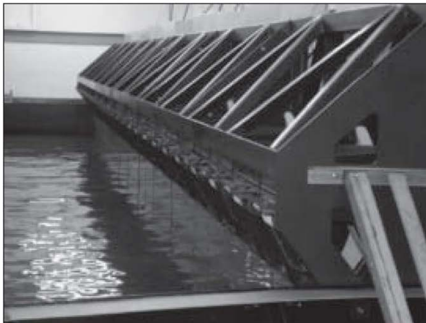
Figure 3. Side view of the wave paddles in the basin of Queen's Univ. Belfast.
