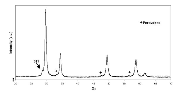
**Fig. 2.** XRD powder pattern of Gd-Ta-O-N after heating GdTaO<sub>4</sub> at 900°C under ammonia flow for 15 h: presence of Gd<sub>2</sub>Ta<sub>2</sub>O<sub>5</sub>N<sub>2</sub> pyrochlore and GdTaON<sub>2</sub> perovskite (weak peaks with +).
