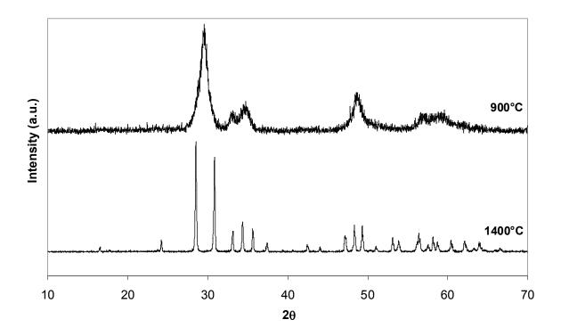
**Fig. 4.** Comparison between the XRD powder patterns of scheelite-type HoTaO<sub>4</sub> (citrate route, 900°C) and fergusonite-type HoTaO<sub>4</sub> (ceramic route, 1400°C).
