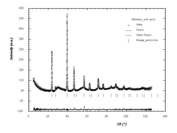
**Fig. 5.** Neutron diffraction powder pattern of the  $YTa(O,N,\Box)_4$  fluorite phase (N wt.% = 4.66).
