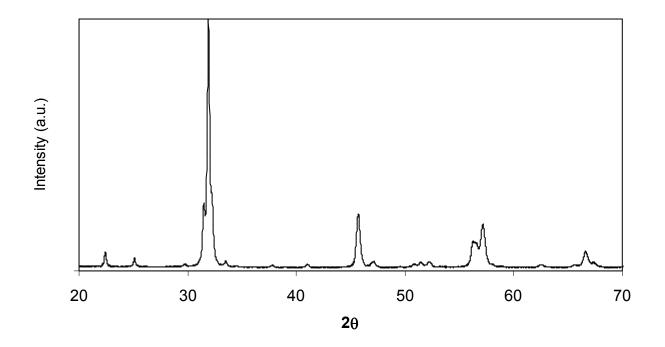
**Fig. 1.** XRD powder pattern of GdTaO<sub>2</sub>N after heating GdTaO<sub>4</sub> at 1000°C under ammonia flow (4x15 h cycle).
