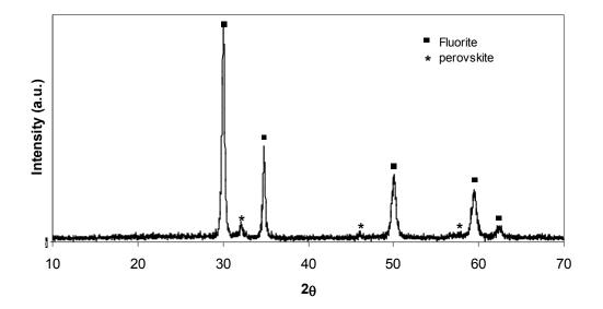
**Fig. 3a.** XRD powder pattern of HoTa(O,N, $\Box$ )<sub>4</sub> after ammonolysis of HoTaO<sub>4</sub> fergusonite at 950°C for 5x15 h.
