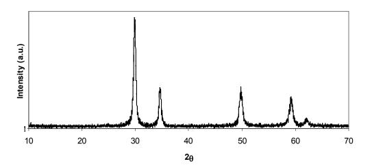
**Fig. 3b.** XRD powder pattern of HoTa(O,N, $\square$ )<sub>4</sub> after ammonolysis of HoTaO<sub>4</sub> scheelite (900° C, 15 h).
