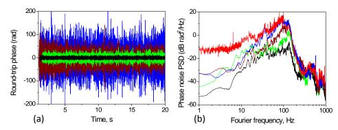
Fig. 4. a) Phase fluctuations along time of each span of the compensated cascaded link (black, green, brown and blue curves for the spans 1 to 4, as depicted on Fig. 1 calculated from the inloop error signal, b) Phase noise spectral density of the successive spans of the cascaded link (same colors as for (a)) calculated from the in-loop error signal (and divided by two) and the whole cascaded link (red curve) calculated from the end-to-end phase signal.
