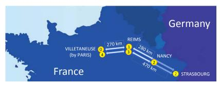
Fig. 1. Scheme of the four-spans cascaded optical link using the RENATER fiber network between Villetaneuse and Nancy, and its extension to Strasbourg.
