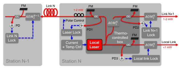
Fig. 3. Schematic of the Nth repeater station, OC: optical coupler, FM: Faraday mirror, PD: photodiode, PC: polarization controller, AOM: acousto-optic modulator.
