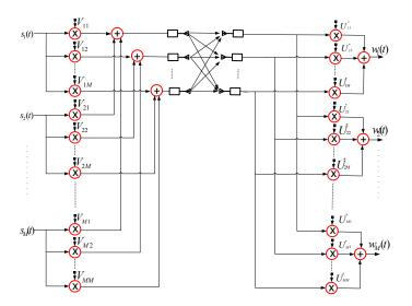
Fig. 1. Spatial-division multiplexing with beamforming technique.
