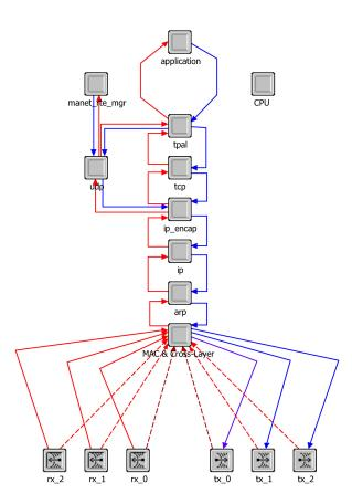
Fig. 5. Node model for MIMOMAX implementation.
