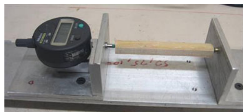
Fig. 3 The fabricated device for measuring longitudinal dimensions in short samples
