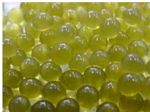
Fig. 1 Immobilization of microbial cells in calcium alginate beads by cross-linking technique
