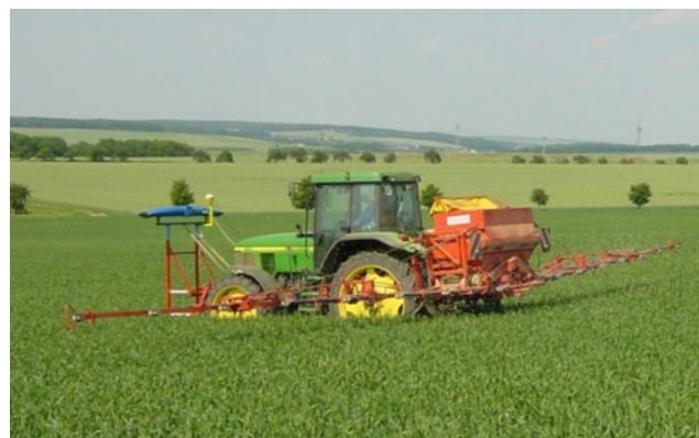
Fig. 3 Implementation of variable-rate technology for site-specific nitrogen application in a winter wheat field in southern Germany (From: Schmidhalter U., Life and Food Sciences Center Weihenstephan of the Technische Universität München)
