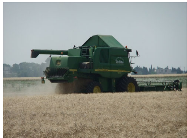
Fig. 4 Precision harvest of durum wheat in southern Italy. The data of yield are recorded with a John Deere combine equipped with a yield monitor system (with grain mass flow and moisture sensors)
