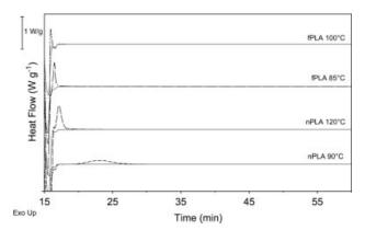
**Figure 3.** DSC thermograms for neat (nPLA) and formulated PLA (fPLA) (black lines) during isothermal cold crystallization at 90 and 120  $^{\circ}$ C for neat PLA and 85 and 100  $^{\circ}$ C for formulated PLA. The baselines, obtained with sapphire at each crystallization temperature, are grey lines. The curves were vertically shifted for legibility.
