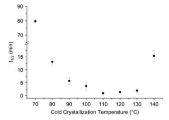
**Figure 2.** Half-time of crystallization of neat PLA (nPLA) as a function of isothermal cold crystallization temperature.
