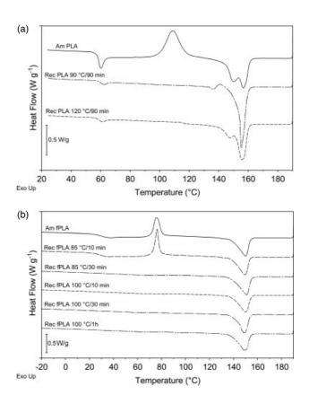
**Figure 4.** DSC thermograms for neat PLA (a) and formulated PLA (b) heated at 10  $^{\circ}$ C min $^{-1}$  after isothermal cold crystallization. The curves are vertically shifted for legibility.
