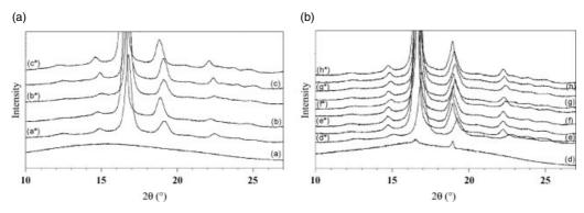
**Figure 5.** WAXD patterns for (a) neat PLA and (b) formulated PLA before and after contact with EA. The labelling corresponds to the notation in Table 1. The samples after contact are noted with an asterisk.
