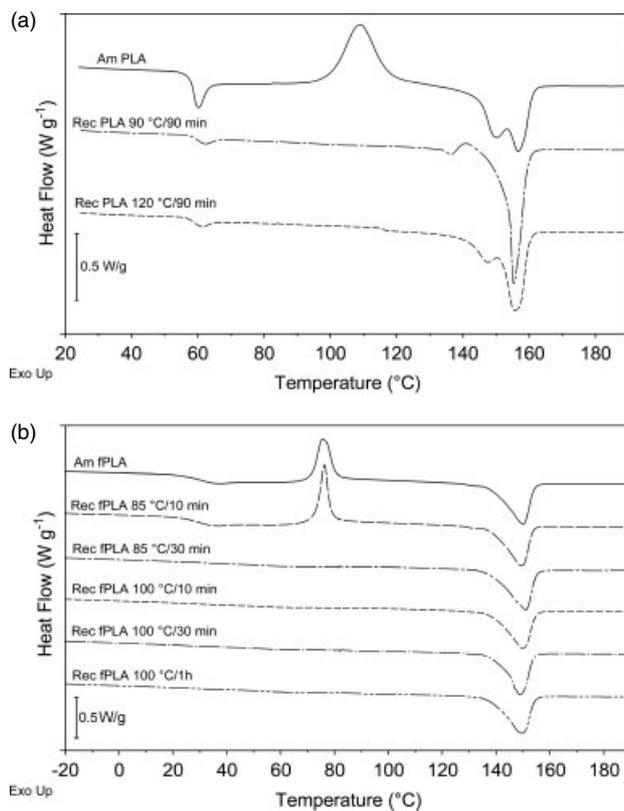
**Figure 4.** DSC thermograms for neat PLA (a) and formulated PLA (b) heated at 10 °C min<sup>-1</sup> after isothermal cold crystallization. The curves are vertically shifted for legibility.
