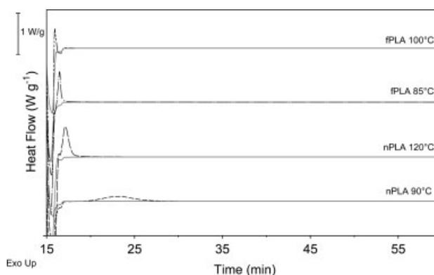
**Figure 3.** DSC thermograms for neat (nPLA) and formulated PLA (fPLA) (black lines) during isothermal cold crystallization at 90 and 120 °C for neat PLA and 85 and 100 °C for formulated PLA. The baselines, obtained with sapphire at each crystallization temperature, are grey lines. The curves were vertically shifted for legibility.
