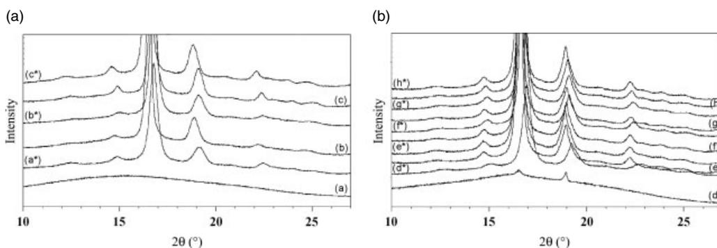
**Figure 5.** WAXD patterns for (a) neat PLA and (b) formulated PLA before and after contact with EA. The labelling corresponds to the notation in Table 1. The samples after contact are noted with an asterisk.
