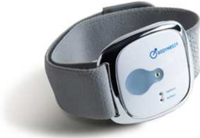
Figure 1: The Bodymedia armband used to record the GSR of participants (illustration from http://www.bodymedia.com/ )
