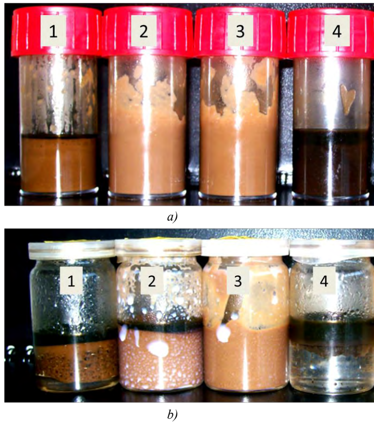
Figure 8 : Emulsions obtained with a blend crude oil (20%vol. and Marcol 52 80%vol). (1: particle-free water; 2: d_p = 280\text{nm} , I = 0.0\text{M} , 3: d_p = 280\text{nm} , I = 0.004\text{M} ; 4: d_p = 280\text{nm} , I = 1\text{M} )
