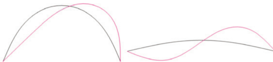
Figure 3. Buckling modes of pre-buckled arches with different rise-over-span ratios (deformed shape in red).
