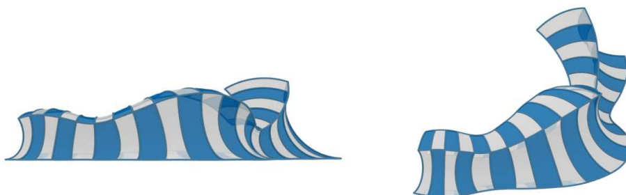
Figure 7: Doubly curved shape with a unique crease as Generalized Cyclidic Net
