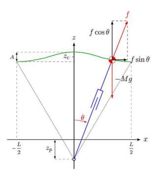
Figure 1: Generalized inverted pendulum in the sagittal plane.
