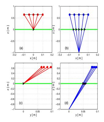
Figure 5: The inverted pendulum motion in sagittal and frontal planes in two cases:  $z_p = 0$  and  $z_p = -1$  m
