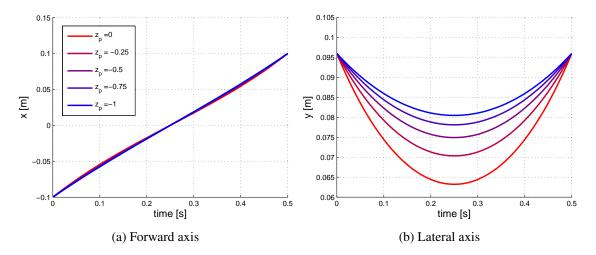
Figure 4: Horizontal trajectory of CoM as a function of time for five values of  $z_p$
