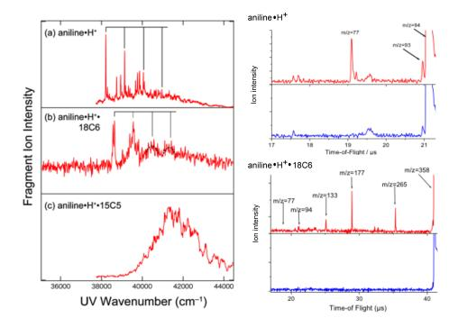
Fig. 1. (left) UVPD spectra: (a) aniline• $H^+$ , (b) aniline• $H^+$ •18C6, and (c) aniline• $H^+$ •15C5. (right) TOF spectra of aniline• $H^+$  and aniline• $H^+$ •18C6, without UV irradiation (blue) and with UV irradiation fixed at the band origins (red). The solid black lines in figure 1a and 1b show the progression with an interval of ~920 cm<sup>-1</sup> assigned to the ring breathing mode.
