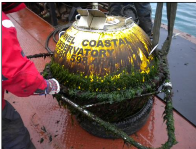
Fig. 2. Heavily fouled directional waverider buoy [20].
