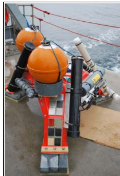
Fig. 5. Material samples attached to instrumentation tripod [28].
