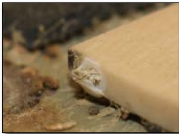
Fig. 6. Barnacle attached to edge of glass fiber composite sample [28].
