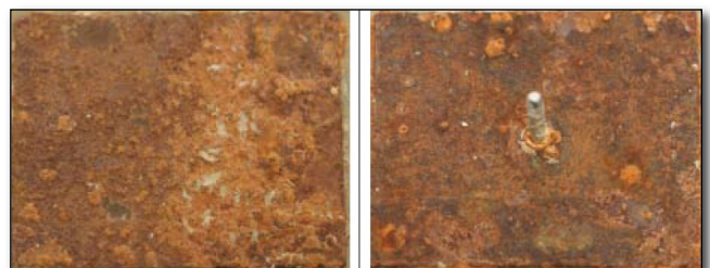
Fig. 10. Common steel coupon corrosion [28].
