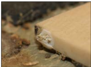
Fig. 7. Barnacle attached to edge of glass fiber composite sample [10].
