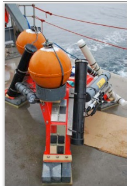
Fig. 6. Material samples attached to instrumentation tripod [10].
