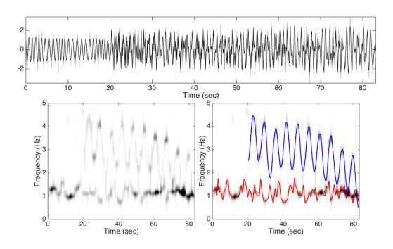
Figure 3: Top: the noisy signal Y is shown as the gray curve with the clean signal f superimposed as the black curve. In the second row, the intensity of the time frequency representation,  $|\tilde{R}_Y|^2$ , determined by our proposed Tycoon algorithm is shown on the left; on the right hand side, the instantaneous frequencies associated with the two components are superimposed on  $|\tilde{R}_Y|^2$  as a red curve and a blue curve.
