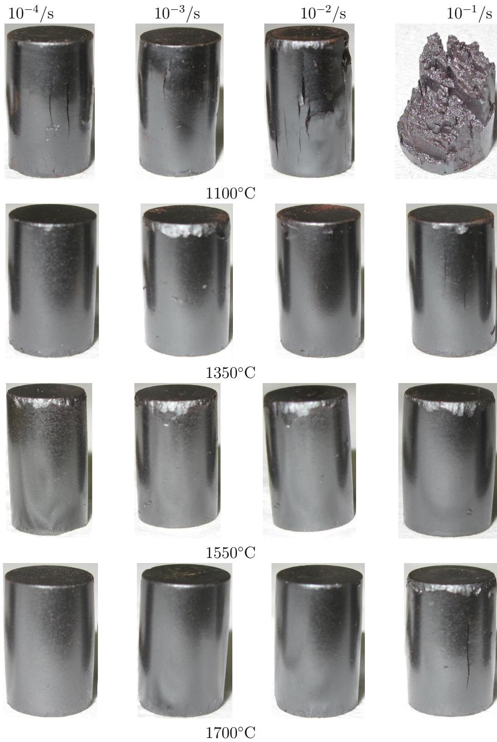
Figure 5: Shape of the samples after the tests.
