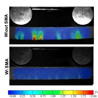
(c) Digital image correlation results of engineering cementitious composite (ECC) beams (508mm in length) with and without SMA reinforcement at the end of 7 loading cycles. Strain fields in the without specimen (top) indicate the presence of microcracks which are greatly diminished by SMA presence (bottom). ©IOP Publishing. Reproduced from [264] by permission of IOP Publishing. All rights reserved.
