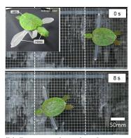
(b) Bioinspired turtle robot constructured using SMA composites as actuators for motion. Top and bottom show the start and finish of a swimming test with the robot displayed in the insert. ©IOP Publishing. Reproduced from [221] by permission of IOP Publishing. All rights reserved.
