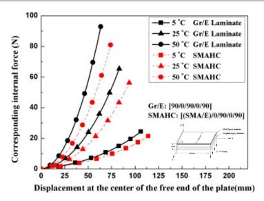
Fig. 19: Actuation response of a hybrid SMA composite presented in terms of deflection at the center of the end edge vs. corresponding internal force. The geometry and boundary conditions of the SMAHC plate are shown as an insert. Reprinted from [97] with permission from Elsevier.
