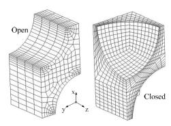
(b) Finite element meshes employed in the analyses of periodic open and closed pore SMA, respectively, containing pore volume fraction of 0.4.
