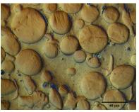
(e) Indium matrix composite with CuAlNi SMA particle reinforcement producing a high damping material. Reprinted from [391] with permission from Elsevier.
