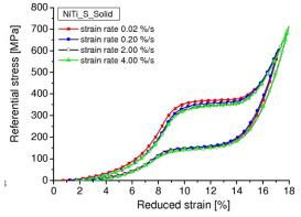
(a) Stress–strain response of a braided, solid NiTi-elastomer composite at different strain rates. ©IOP Publishing. Reproduced from [176] by permission of IOP Publishing. All rights reserved.
