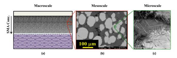
Fig. 10: Multiple scales of interest in the analysis of SMA composite materials: (a) Macroscale-A functionally graded, hybrid composite for extreme environments<sup>2</sup>; (b) Mesoscale-A NiTi (white gray)  $Ti_2AlC$  (darker gray) with heterogeneous microstructure, porosity (black), and reaction layers (Reprinted from [187] with permission from Elsevier); and (c) Microscale-Martensitic twins and accompanying nanoprecipitates of a NiTi<sup>3</sup>.
