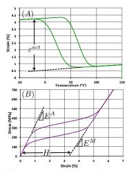
(b) (Top) Actuation (isobaric cooling heating cycles) response under a constant 100 MPa load and (bottom) the pseudoelastic response
