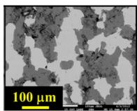
(c)  $NiTi - Ti_3SiC_2$  composite produced via spark plasma sintering. Reprinted from [187] with permission from Elsevier.
