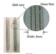
(a) Polymer matrix composite reinforced with smart SMA weave in insert. SMA wires are used as warp fibers while carbon fibers take the weft position thereby improving shape retention possibilities. ©IOP Publishing. Reproduced from [453] by permission of IOP Publishing. All rights reserved.
