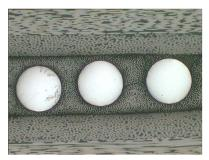
(a) Carbon/epoxy matrix reinforced with small diameter (0.25 mm) NiTi wires. Reprinted from [488] with permission from Elsevier.
