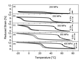
(b) Actuation response (strain—temperature under a constant stress), under different applied loads of a braided, hollow NiTi-elastomer composite. ©IOP Publishing. Reproduced from [176] by permission of IOP Publishing. All rights reserved.
