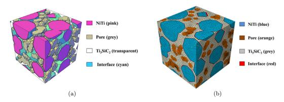
Fig. 18: Detailed 3D, multiphase (a) numerical microstructure and (b) finite element mesh used for the thermal analysis of a NiTi - Ti<sub>3</sub>SiC<sub>2</sub> composite. Reprinted from [93] with permission from Elsevier.
