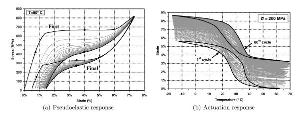
Fig. 4: Evolution of characteristics SMA responses over repeated cycling (training). Taken from [169].
