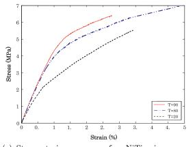
(c) Stress–strain response of a NiTi wire-epoxy composite at different temperatures (wire  $A_f$  is 65° C). Reprinted from [348] with permission from Elsevier.
