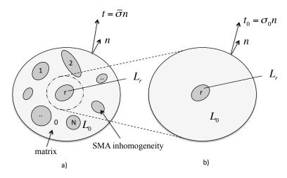
Fig. 12: Illustration of the boundary value problem considered for analysis via Eshelby-based mean field approaches: (a) a composite comprised of N distinct, ellipsoidal inhomogeniety phases embedded in a distinct matrix and (b) the Mori-Tanaka problem for the r-th phase. ©IOP Publishing. Reproduced from [252] by permission of IOP Publishing. All rights reserved.
