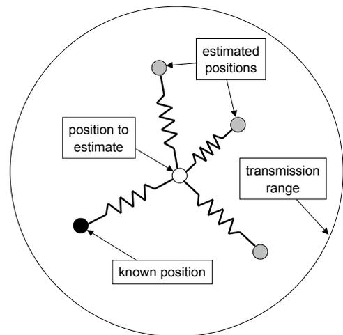
Figure 2: Bond model for positioning.
