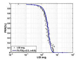
Fig. 6. Fitting LQI averaged over links.
