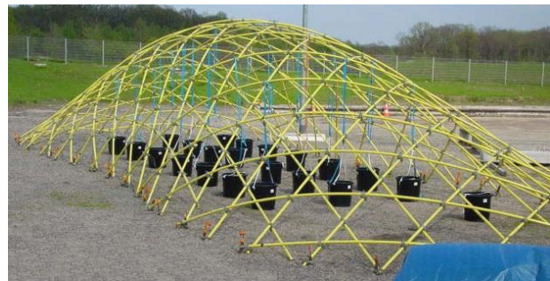
Figure 6: First experimental gridshell under testing.
