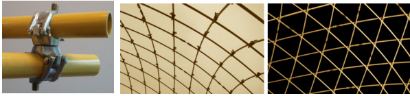
Figure 8: Left: Joint detail. Centre: Mesh before bracing. Right: Mesh after bracing
