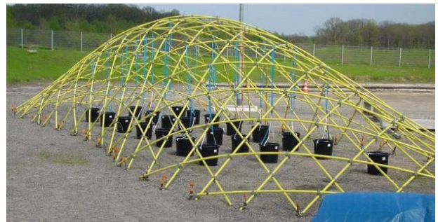
Figure 6: First experimental gridshell under testing.
