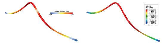
Figure 8: deformed shape from custom plugin
