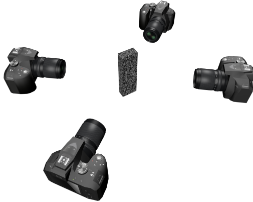
Figure 1: Schematic drawing of a stereovision setup with a multisurface object (parallelepiped) in the center observed by a four-camera system. This elementary example will be used in Section 4 to illustrate the proposed methodology.
