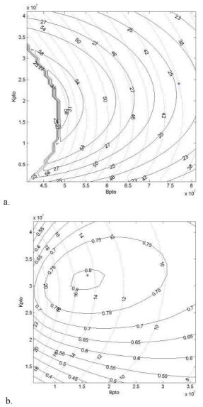
Fig. 7 Contour plots of the power recovered per unit length (solid lines) and of the maximum angle of oscillation (dotted lines) of the flap converter, depending on PTO parameters.
