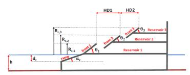
Fig. 4 Sketch of a 3-level SSG structure.
