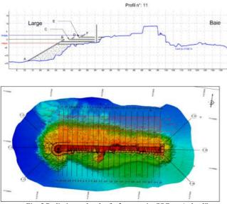
Fig. 5 Preliminary sketch of a 3 reservoirs SSG on Artha dike
