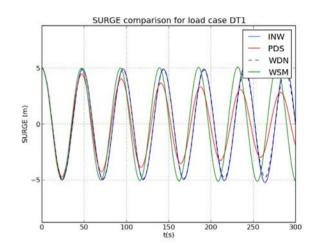
Figure 9. Comparison of surge motion for load cast DT1.
