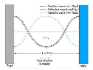
Figure 7. Wave radiation at a frequency of 1.66 rad/s resulting in wavelengths of  $\lambda = L$ .
